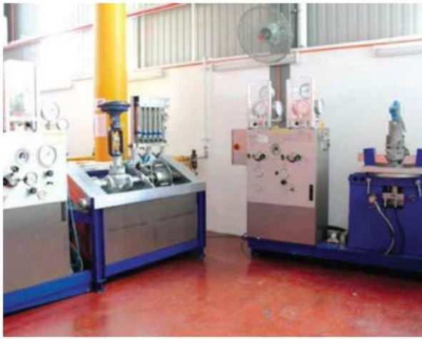
Control & Safety Valve Test Bench (1/2" - 16")
